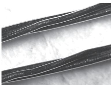
Fig. 5. Steel cord 3x0,30 HT FRP appearance
