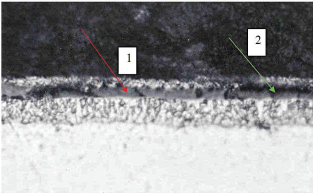
Fig. 4. Microstructure of a TiC – coating formed by the CVD method, featuring a brittle  $\delta$ -phase (red arrow 1) in the form of isolated inclusions and bands appeared in the surface zone in the result of local decarburization. Green arrow 2 points to a crack in the sub-surface band of a  $\delta$ -phase formed in the result of a high brittleness this phase. x1000
