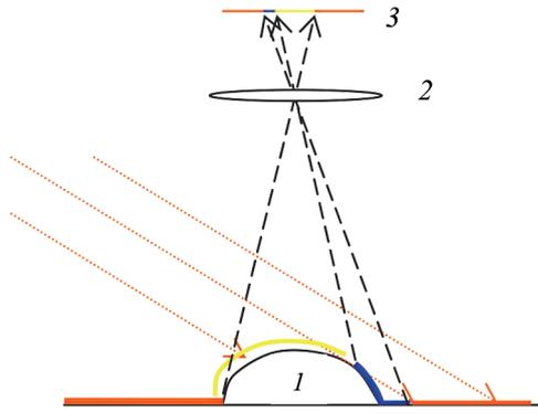
Figure 4. To explanation of formation of an image of a defect at oblique illumination: 1 – defect on the surface; 2 – digital camera lens; 3 – image plane; illuminated and shade sections are marked with yellow and blue colors, respectively
