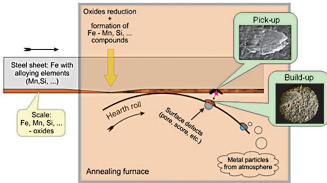
Figure 1. Formation of pickup and build up between steel strip and roll surface
