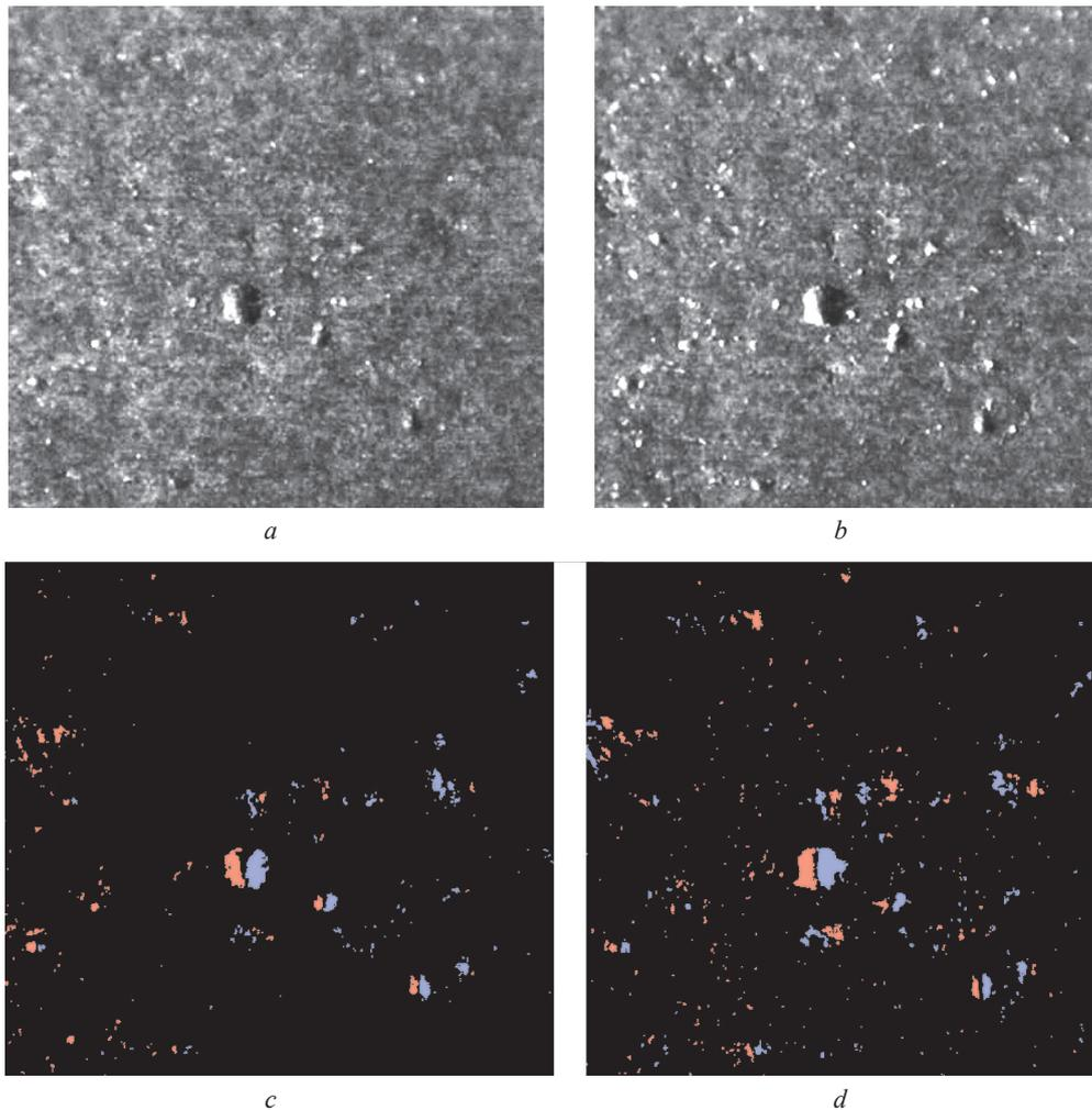
Figure 6. Initial images (*a, b*) at different angles of left-side illumination and artificial synthesized images (*c, d*). Sections with higher brightness at left light incidence and with lower brightness at right-side illumination are marked with red color. And vice versa are marked with blue color, respectively. Incident angles are 45 degrees (*a, c*) and 65 degrees (*b, d*)
