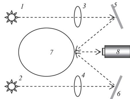
Figure 5. Measurement scheme with two illumination channels: 1, 2 – illuminating lamps; 3, 4 – condensers; 5, 6 – reflecting flat mirrors; 8 – recording digital camera; 7 – roll under study
