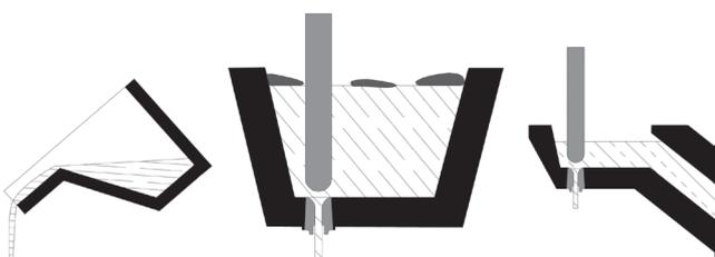
Fig. 3. Tilting ladle, Stopper ladle, Pressurized pouring system
