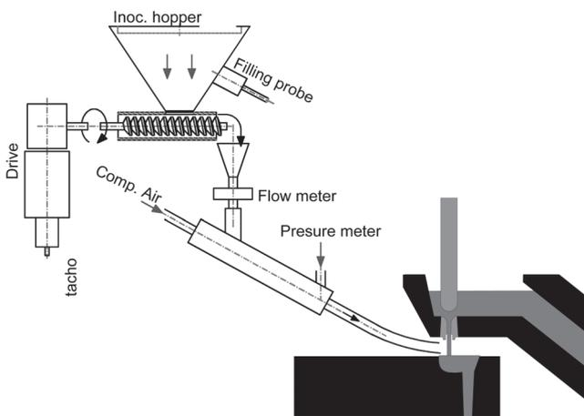
Fig. 8. Pouring Stream Inoculation Monitoring System
