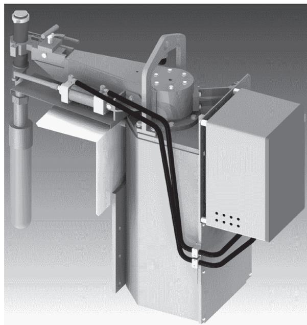
Fig. 6. Design of the ABP stopper system for automatic pouring
