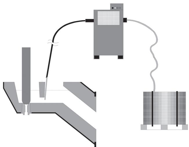
Fig. 9. Wire Inoculation Configuration
