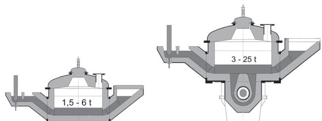
Fig. 4. The unheated Pouromat® System and the Heated Presspou® System
