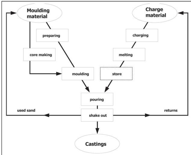
Fig. 2: Simplified Diagram: Principal Material Flow Circuit
